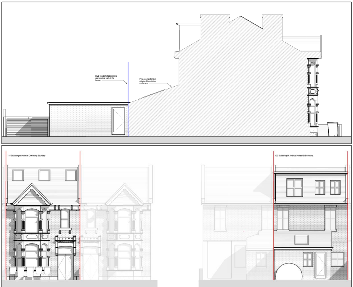
Figure 1 Proposed Elevations showing extensions and rooflights
