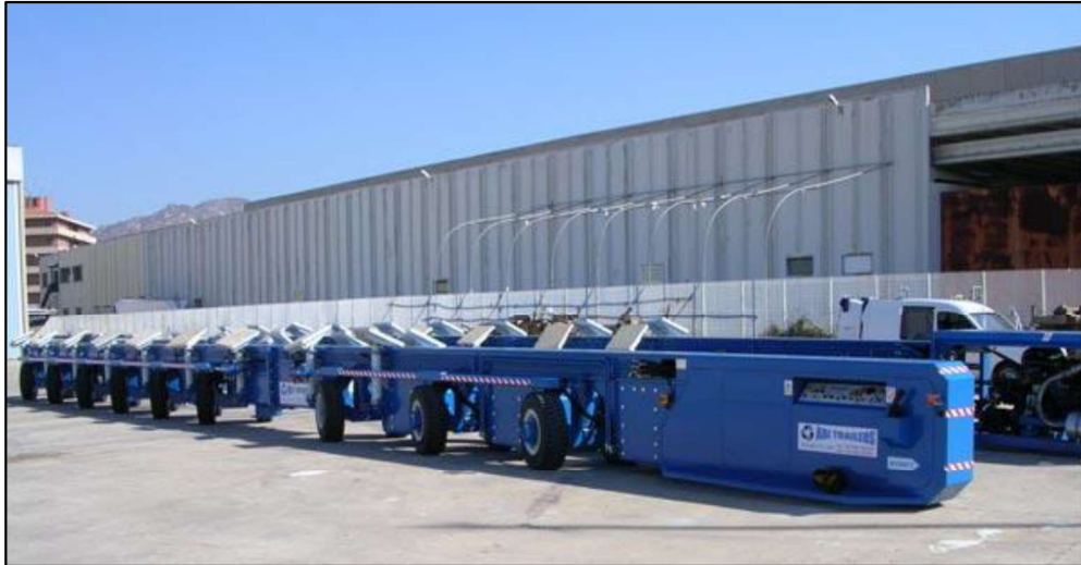
Figure 4.1 - 300 Ton boat mover to enable efficient use of storage space and increase vessel storage capacity
