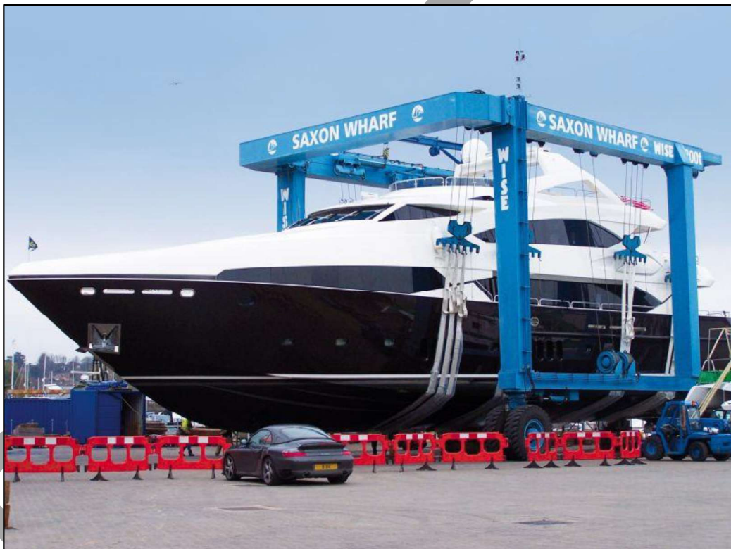
Figure 3.1 - Vessel supported on individual lifting strops Saxon Wharf
