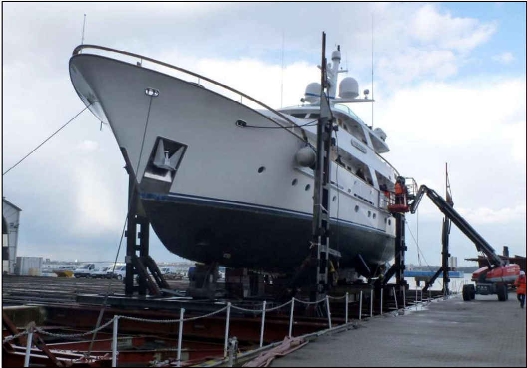
Figure 3.2 - Vessel on the slipway cradle at Solent Re-fit
