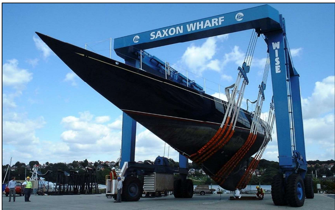
Figure 4.1 J Class Mast Removed Due to Air Height Restrictions – River Itchen Southampton
